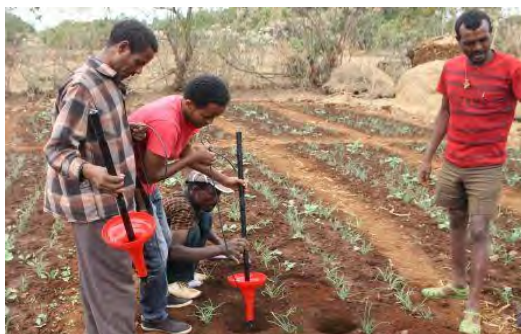
Figure 6: Installation of Wetting Front Detector, Dangishta, Ethiopia
