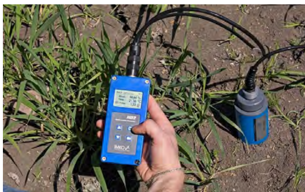
Figure 8: Use of Time Domain Reflectometry to Find Volumetric Moisture Content of Soil
